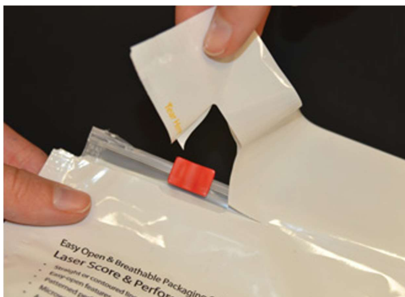
Figure 12: Contour laser-score line added to an easy-open zipper pouch.
