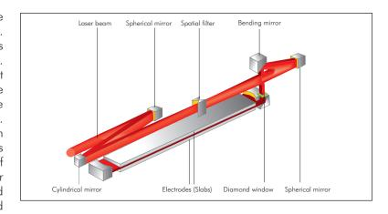
service are eliminated. Thus, optics integrated into the resonator that are contaminated by flowing laser gas (especially the outcoupling windows) are a thing of the past.
