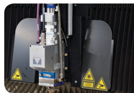
Cutting head with motorized focal lens
