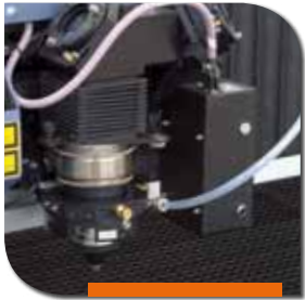
CCD kit for register cutting with print marker recognition
