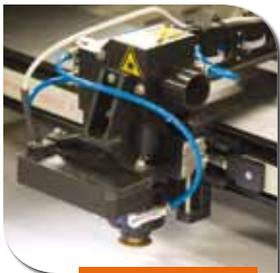
CCD camera kit for registration of cutting to printing markers
