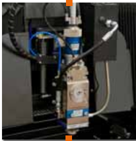
Cutting head with capacitive sensor
